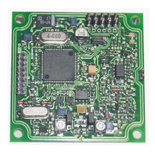
Multitag proximity reader module for identification of Smart Labels in the fields of application retail, industry, logistics etc.
